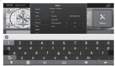
It provides virtual keyboard input mode. In the process, you can choose character by moving cursor, and press **ENTER** to complete character input. At the same time, you can change the input mode from virtual keyboard.
